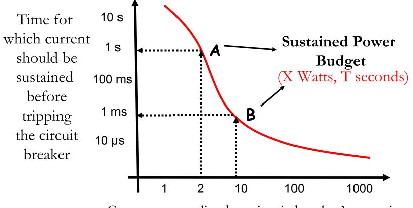
Current normalized to circuit-breaker's capacity
