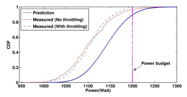
Provisioning for the 90<sup>th</sup> percentile power needs: Threshold
