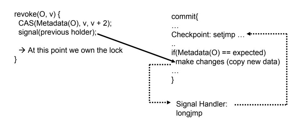
How to synchronously signal ? We use a custom signalling service implemented as a kernel module
